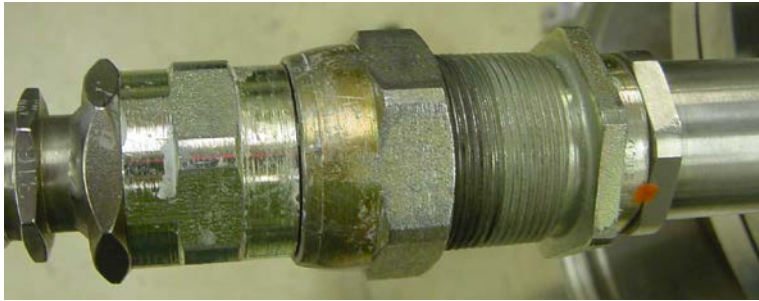
Figure 3 Female to male connection, hand tightened
