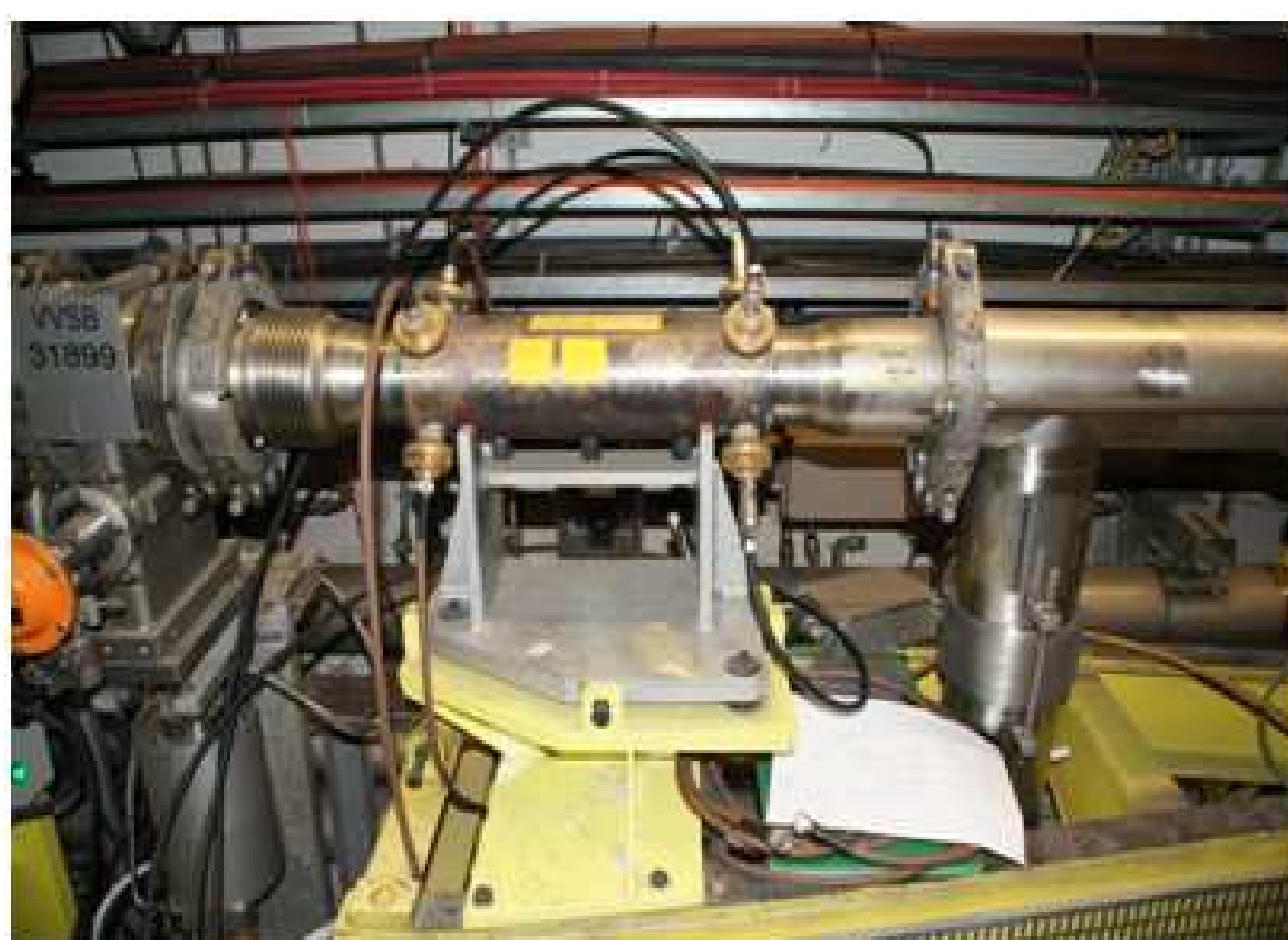
Figure 7: An exponentially-tapered pickup array (BPW 319.01) is used as a kicker in the tunnel for our MD measurements. A similar array (BPW 321) is used as a pickup.
