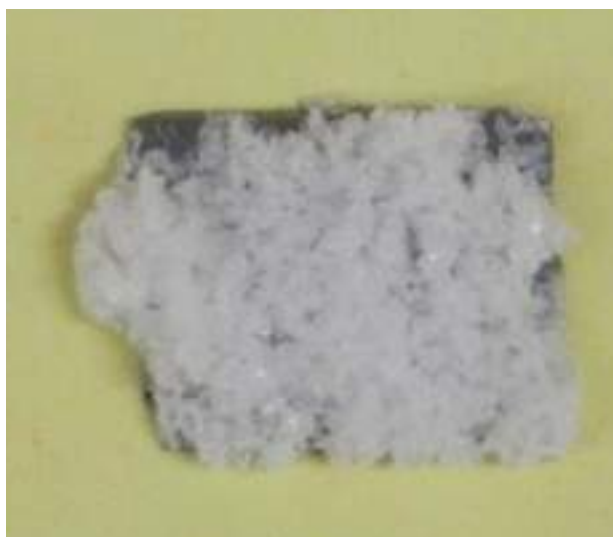
Figure 1. Photo of the simple NaCl reflector made by dabbing a supersaturated slurry of NaCl and \text{H}_2\text{O} onto a Si wafer piece (area \approx 1 \text{ cm} \times 0.8 \text{ cm} ). The NaCl was taken from a 13 oz. container of un-ionized Diamond Crystal Kosher Salt purchased at Andronico's Market in \approx 2009 . (July 23, 2012)
