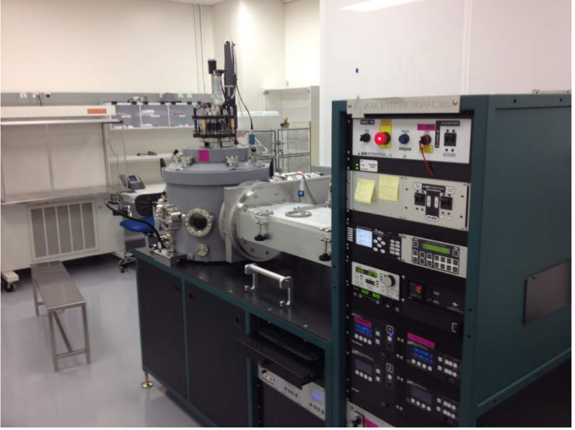
Figure 4.2: AJA International ATC-2200 confocal DC/RF magnetron sputtering system used for the deposition of W and Al films in this work. The system allows us to vary Ar pressure, sputtering target power, and substrate bias voltage to adjust properties of our films, including W Tc.
