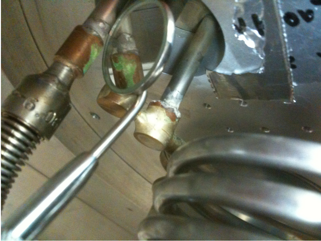
Figure A-7. Visual appearance of a connection that had a helium leak. The green is a result of acidic flux that was never properly cleaned during fridge installation. Over time it is believed this corroded the connection to the point that a leak appeared. This was repaired by the machine shop re-flowing the solder. This particular line is on the condensing circuit. Courtesy of Durdana Balakishiyeva.
