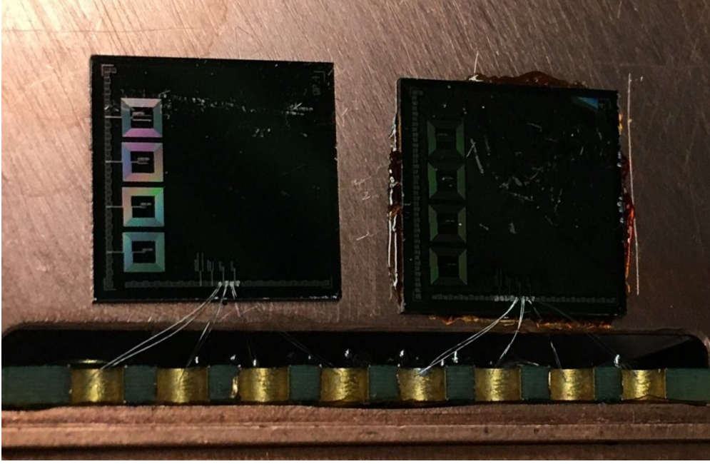
Figure 5.8: (Left) The QP.4 chip with the 25\,\mu\text{m} \times 100\,\mu\text{m} \times 40\,\text{nm} and 50\,\mu\text{m} \times 200\,\mu\text{m} \times 40\,\text{nm} rectangles being read out, which is simply resting on the Cu housing. (Right) The QP.4 chip with the 25\,\mu\text{m} \times 100\,\mu\text{m} \times 40\,\text{nm} and 50\,\mu\text{m} \times 200\,\mu\text{m} \times 40\,\text{nm} rectangles being read out, which is glued to the Cu housing with GE-7031 varnish. Photo by William Page.
