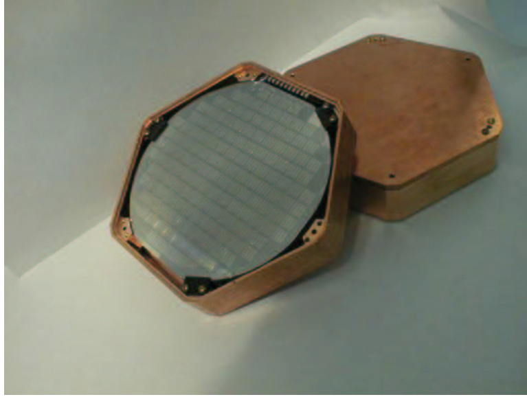
Figure 4.1: A photograph of a ZIP detector in its housing. The exposed surface shows the phonon sensor pattern.
