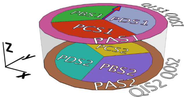
Figure 1.8: Layout of SuperCDMS phonon and charge sensors. Each side has three pie wedge shaped phonon sensors and a ring shaped channel around the outside, and two charge sensors. The alignment is rotated by 180 degrees between the sides. [47]
