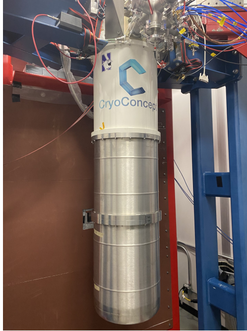
Figure 6-2. The dilution refrigerator system used in HVeV Run 4. The HVeV detectors are housed inside the refrigerator.
