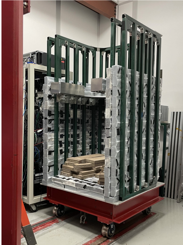
Figure 5-3. The lead shielding used at NEXUS. During HVeV Run 4, these lead bricks surrounded the CryoConcepts dilution refrigerator to reduce gamma radiation. Polyethylene boards are also visible in the setup, providing additional shielding against neutron radiation.
