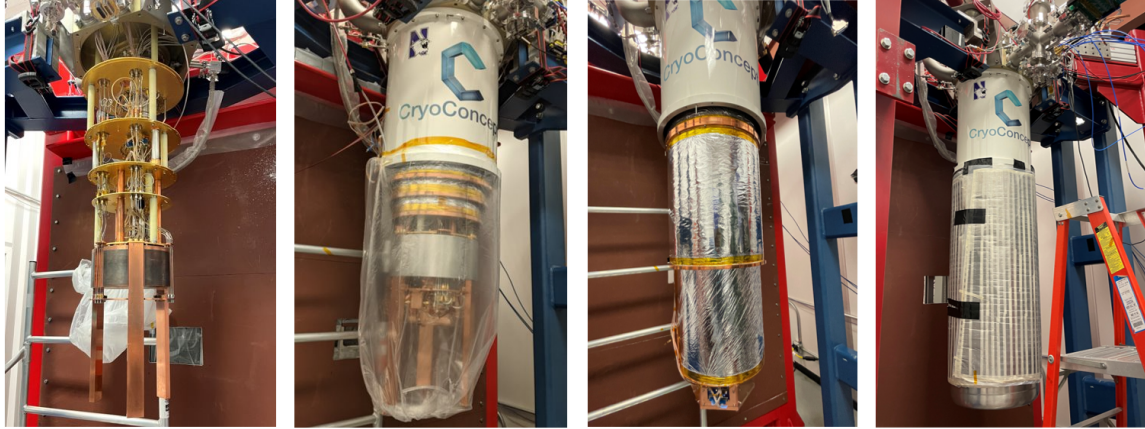
Figure 3.3: Various components of the cryogenic refrigerator modeled in Geant4 simulations. From left to right: copper stages, the assembled fridge without nested vessels, with one of the internal vessels, and the full assembly including the OVC.
