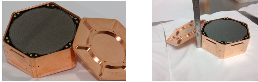
Figure 2.2: SuperCDMS SNOLAB detectors showing an HV detector (Left) and iZIP detector (Right) inside copper housing [2].
