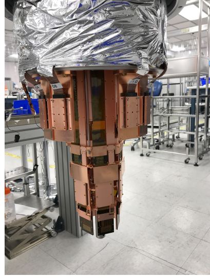
(b) The detector tower installed into the Bluefors fridge.
