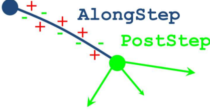
Figure 3.1: Illustration of a color-coded G4Step . The blue indicates the AlongStep section in which the continuous processes are modeled. The green indicates the PostStep in which kinematic changes from the production of secondaries are modeled. Figure adapted from Ref. [36].
