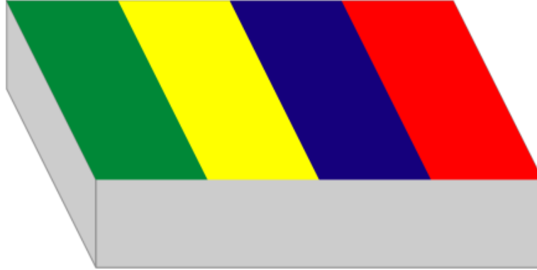
Figure 2.6: Cartoon of detector geometry used in a simple simulation to show that the detector's position response can be linearized. The metal surface is parsed into four sections: the left-outer (green), left-inner (yellow), right-inner (blue) and right-outer section (red).
