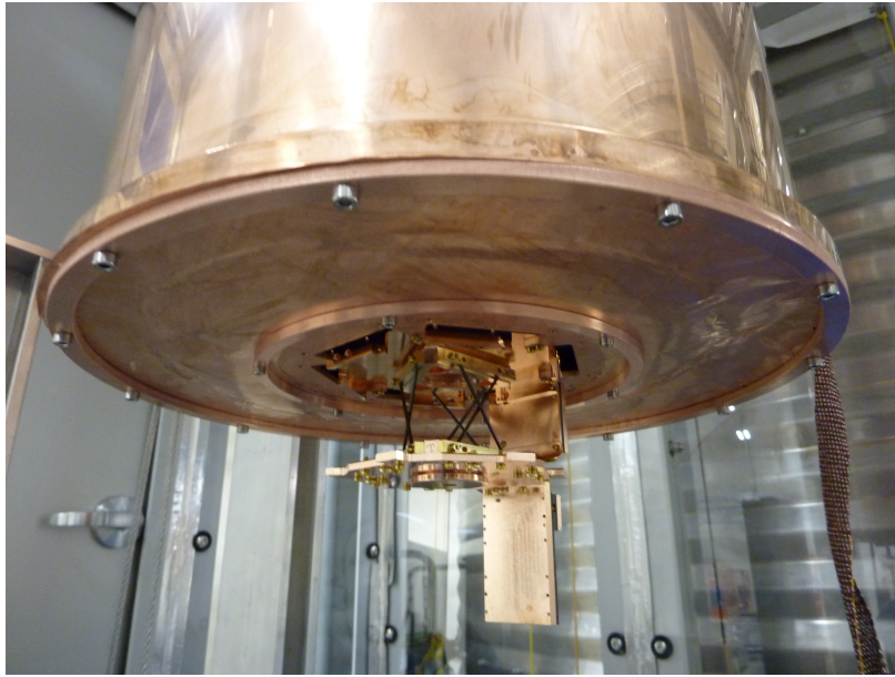
Figure 5.6: Photograph of the copper membrane that provides infrared shielding and heat sinking for the still stage of the tower. The membrane attaches to the tower stage by a copper adapter plate and ring, and attaches to the bottom edge of the still can with a larger diameter ring.
