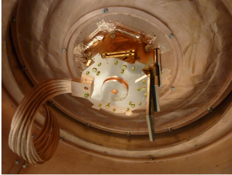
Figure 5.7: Photograph of the copper strap that connects the 4 K stage of the tower to a rim on the inside of the 4 K can. With the new Ti VFC, this strap now connects to the bottom of the still can.
