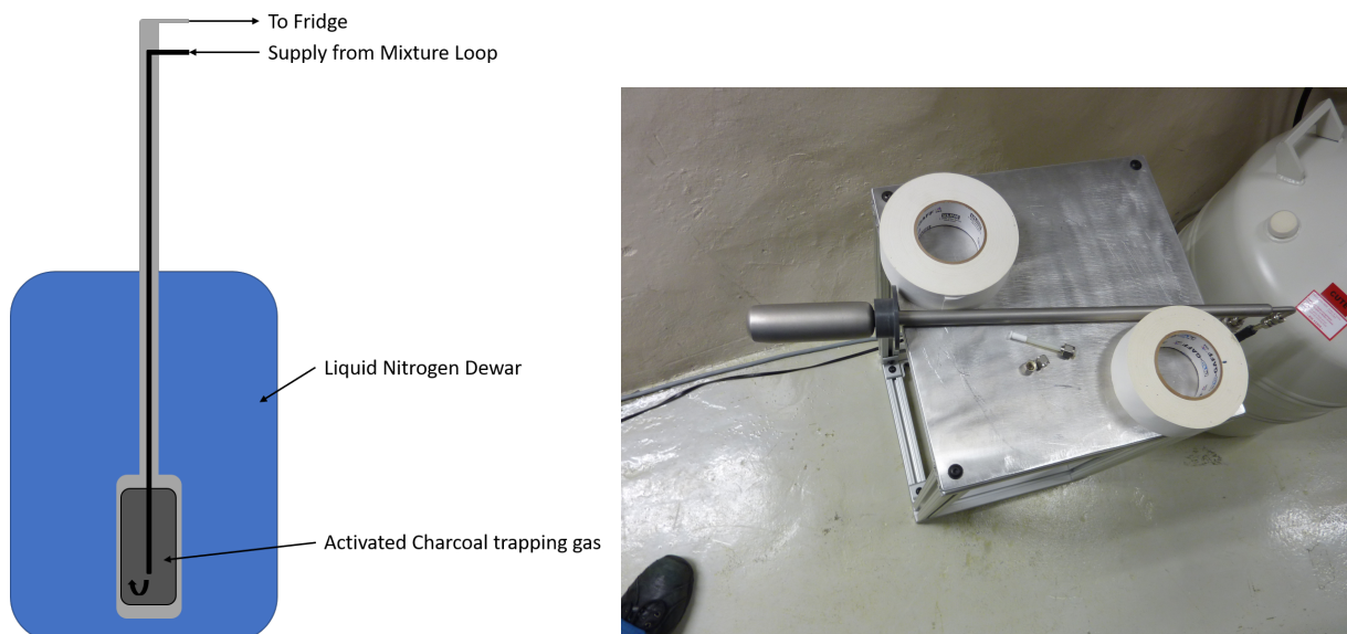
Figure 4.7: (Left) Schematic of a typical cold trap setup using cocentric tubes for the in/out flow with the transfer between the tubes occurring at the bottom bulb with activated charcoal which is submerged in Liquid Nitrogen, precipitating any contaminant in the gas into the charcoal. (Right) The Cold Trap used in CUTE resting on a side table for cleaning between runs.
