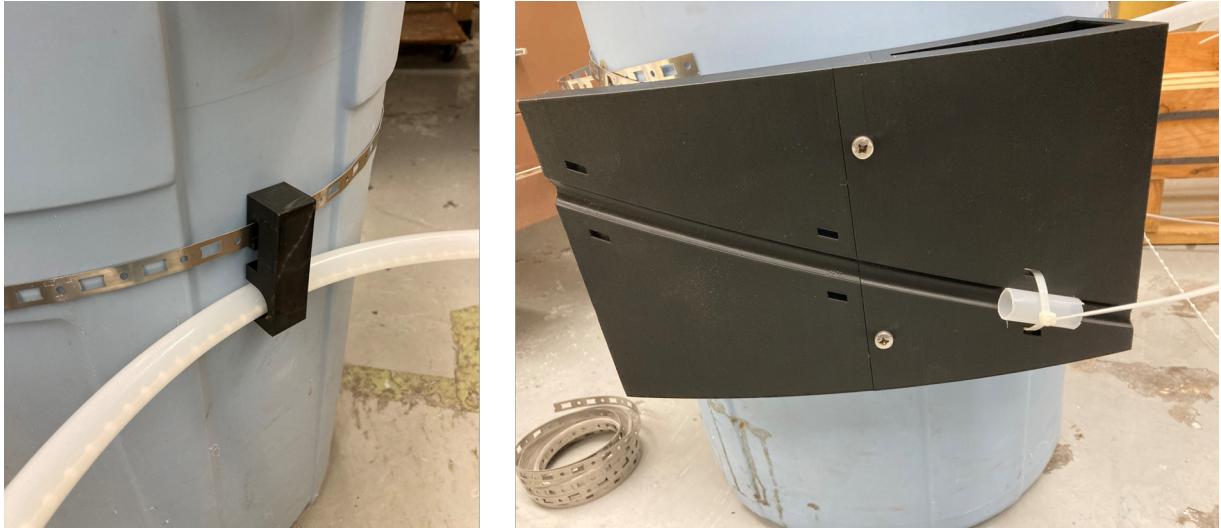
Figure 7.14: Test conditions after the construction of various pieces in the Queen’s lab. (Left) Wormdrive band holding the drywell attachment piece which holds the source tube against the drywell with minimal water separation. (Right) Neutron energy spectrum variation wedge with a sample piece of tubing held in place on it, mounted to a test cylinder using a wormdrive band loop.
