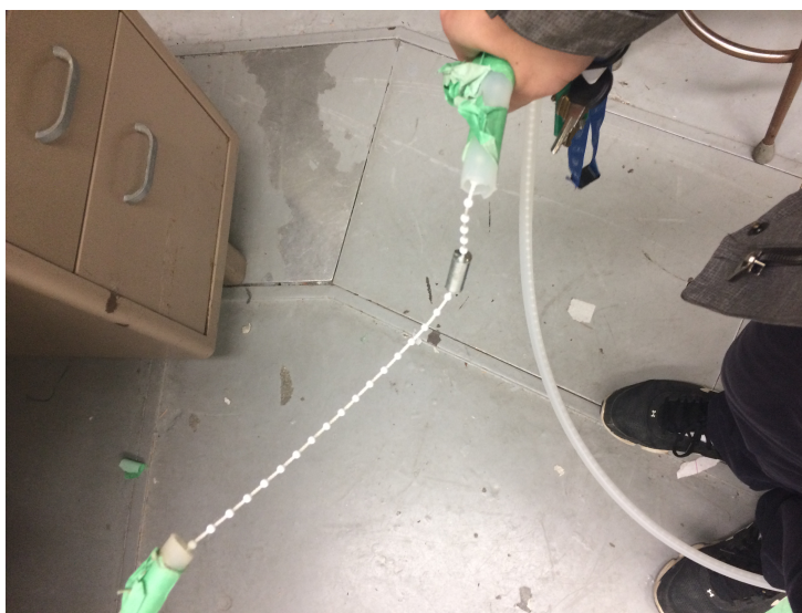
Figure 7.13: Photo of the mock source in place in the testing set up. The chain was loaded in the plastic tube and was attached at both ends to the mock source. The exposed chain was then looped over the stepper motor gear and held in place to prevent skipping and using a protoboard, power supply, and function generator the stepper motor was driven moving the source within the tube.
