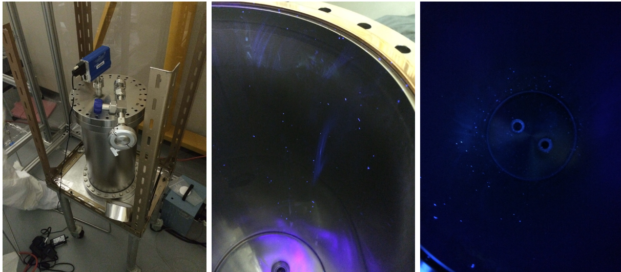
Figure 4.4: Left: Small emanation chamber, with bolts removed, in the HEPA-filtered cleanroom tent. Middle: Inside of emanation chamber, without the black-out cloth, shown with UV light illuminating dust, dirt, and lint inside the S.E.C.. Right: S.E.C. after cleaning the surface with IPA, using lint-free wipes, and finally applying nylon brushes from bottom to top. Some dust remains in the chamber even with vigorous wiping and scrubbing.
