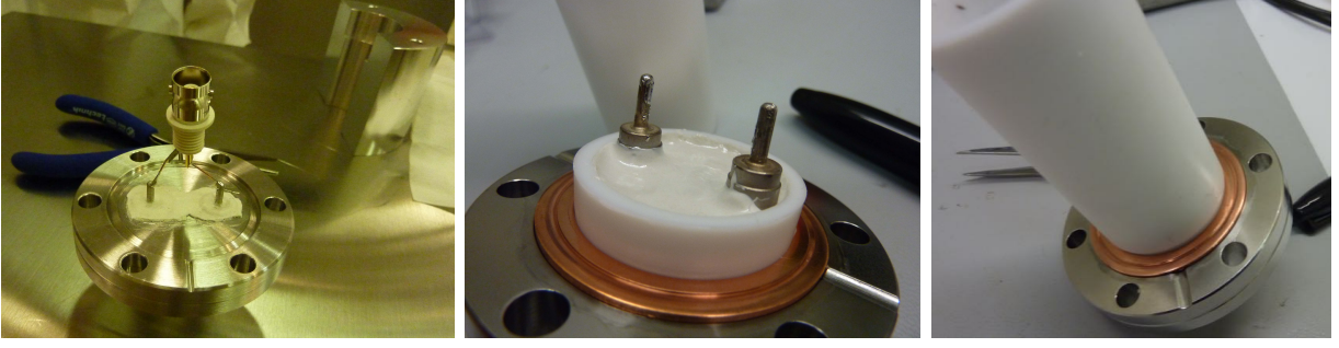
Figure 4.17: Left: First attempted configuration of epoxy potting for the high-voltage feedthrough. This configuration failed to provide sufficient insulation between the high voltage of the electrodes coming from the signal feedthrough. Middle: Second configuration of epoxy potting formed by mixing two-part epoxy paste and evacuating the paste during the curing process. This configuration reduced the arcing somewhat at pressures above 1 Torr. Right: Tubular teflon stand, lathed to fit snugly inside the copper gasket of the high-voltage feedthrough and aluminum gas displacers. This teflon, along with the second configuration of epoxy significantly reduced arcing at pressures P \approx 2\text{--}25 Torr from the 2 kV signal wires to the grounded half-moon stands and feedthrough.
