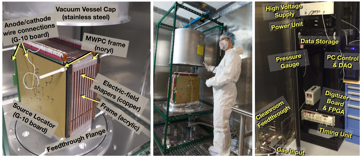
Figure 7.1: Left: The ProtoCage demonstration screening time projection chamber without readout wires following installation in the reduced-radon cleanroom at SDSM&T. The (40 \times 40 \times 20) \text{ cm}^3 TPC is made with an acrylic frame, copper electric-field shapers, and noryl MWPC frames. The TPC itself sits atop a feedthrough flange underneath a vessel cap during operation. The trigger and bulk MWPC frames (noryl) are each strung with a single anode plane sandwiched by 2 cathode planes. To achieve proportional avalanching in the anode grid, the anode and cathode grids are separated by 5.08 mm with a voltage separation V_{\text{MPWC}} \sim 2 \text{ kV} . The wire planes each have 79 sense wires spaced s = 5.08 \text{ mm} apart. Two square G-10 boards (yellow) protect the sense wires and, on the visible side, help to consistently aim calibration sources. The (acrylic) frame separates the trigger and bulk MWPCs by z_{\text{drift}} = 20 \text{ cm} and holds the (copper) electric-field shapers. Middle: The ProtoCage TPC wired with 6 channels of readout from the trigger MWPC. I am using the wench system to place the cap over the vacuum vessel. For now, the ProtoCage data readout consists of many fewer channels (6) than the planned BetaCage configuration, with an active area \approx 3 \times larger. Right: ProtoCage data acquisition system (DAQ), electronics rack, and control PC. The rack has a pressure gauge indicating the inner vessel pressure, a computer with solid-state disk drives for data storage, a high voltage supply, a timing unit to control the digitization rate and a field programmable gate array (FPGA) which digitizes and records the pulses to send to the computer.
