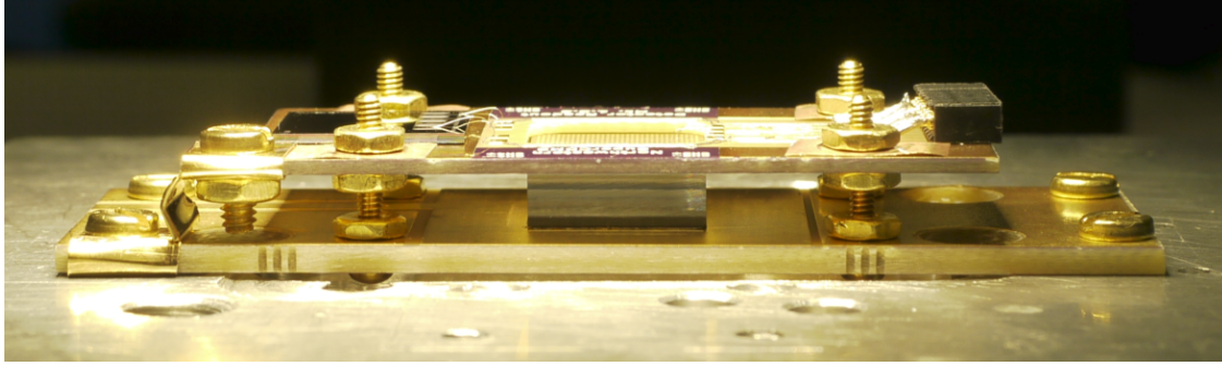
Figure 3-4. The sideview of the HVeV detector in its holder. The detector chip is pinned between two PCBs. A keen eye might notice the black strip on the left side of the top PCB. This was a secondary detector which is meant to be used for background rejection but was not used in this run due to the operating temperature being too close to that detector's superconducting transition temperature
