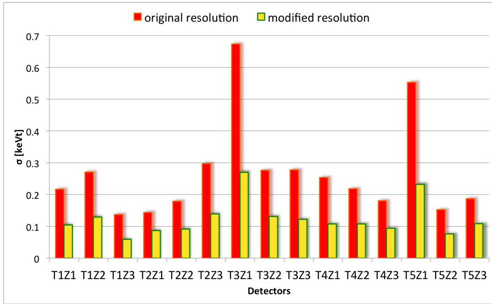
Figure 5.8: Distribution of phonon base-line energy resolution ( \sigma ) of various iZIPs calculated in the optimum filter framework. The three iZIPs with best resolution are T1Z3, T2Z1 and T5Z2 with \sigma = 138, 144 and 153 \text{ keV}_t respectively.
