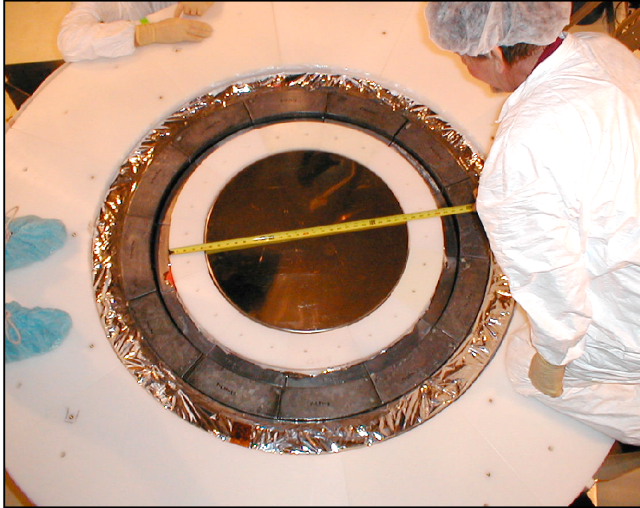
Figure 3.6: Top view of the (closed) CDMS icebox. The upper sections of the shield have been removed to facilitate access (cf. Figure 3.5).
