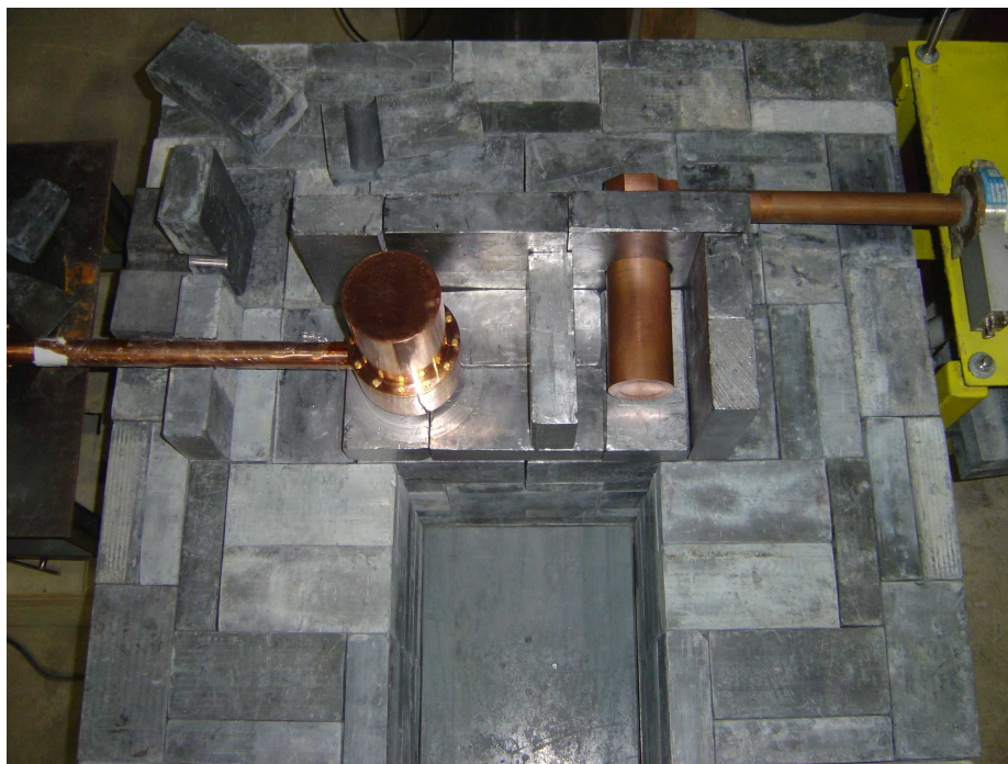
Figure 10.6: Partially reconstructed GATOR (left) and Diode M (right) chambers during the November 2005 repair operation.
