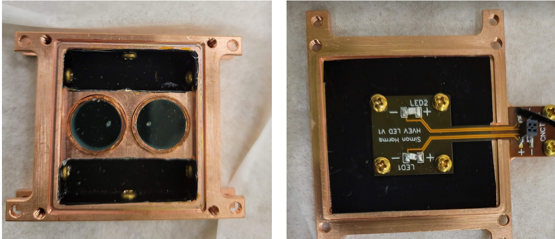
(a) Bottom side of an LED box showing two pinholes each covered with an IR filter. (b) The top of an LED box, showing the wiring used to pulse each LED independently.
