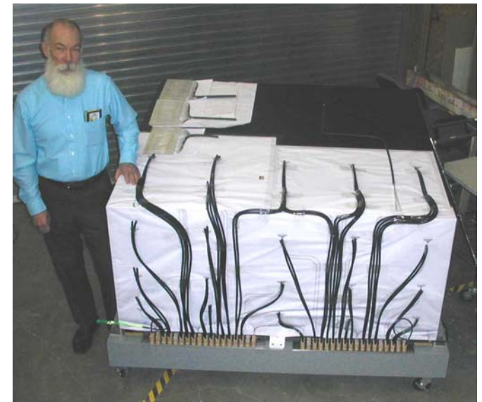
Full-scale mock-up of ACD being used for tile placement and fiber routing
