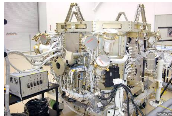
GLAST S/C bus waiting for LAT installation at General Dynamics. GBM installation in progress.
