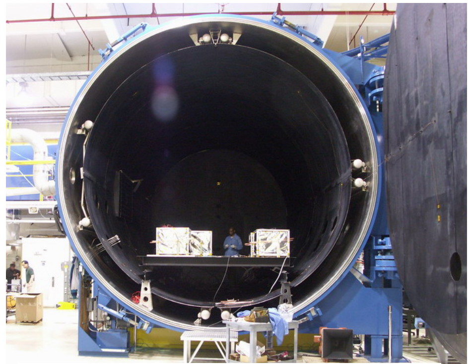
Last 4 CALs (in thermal shields) installed in “Big Blue” TVAC at NRL.
