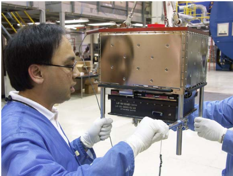
Preparing CAL #18 and flight qual TEM/TPS for thermal vacuum testing
