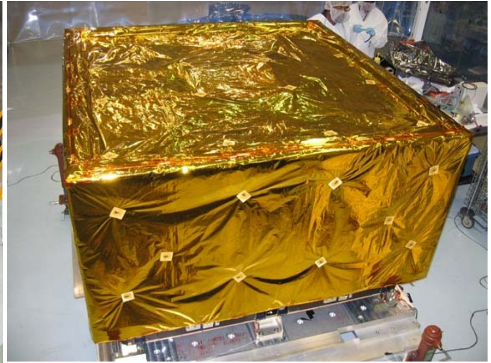
ACD with Micrometeoroid Shield and Multi-Layer Insulation (but without Germanium Kapton outer layer)
