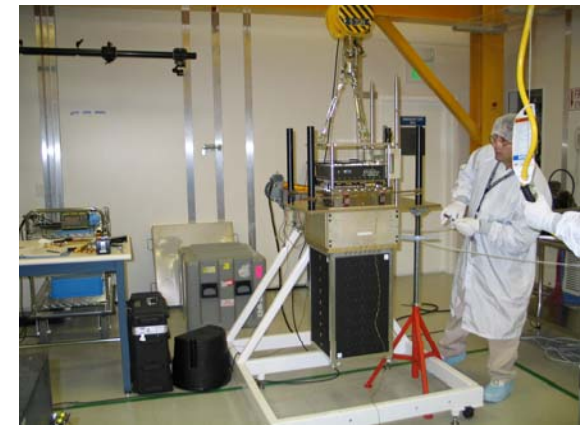
Tower A Assembly CAL/TEM Integrated with TKR A
