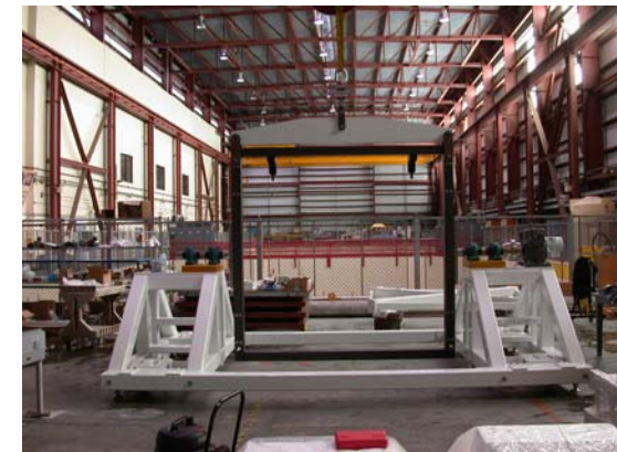
4x4 Z-axis Horizontal Lift Fixture Proof Test Complete
