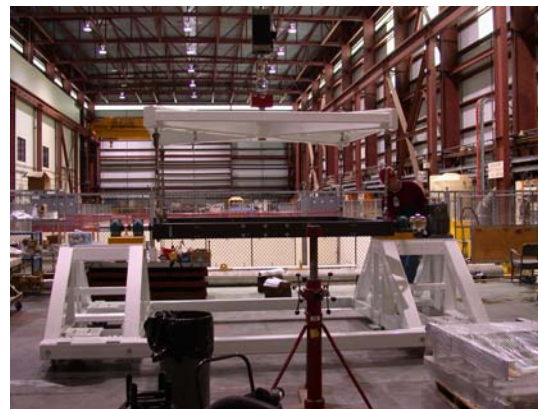
4x4 Z-axis Vertical Lift Fixture Proof Test Complete
