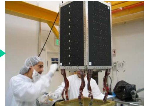
Installing into the single bay test stand
