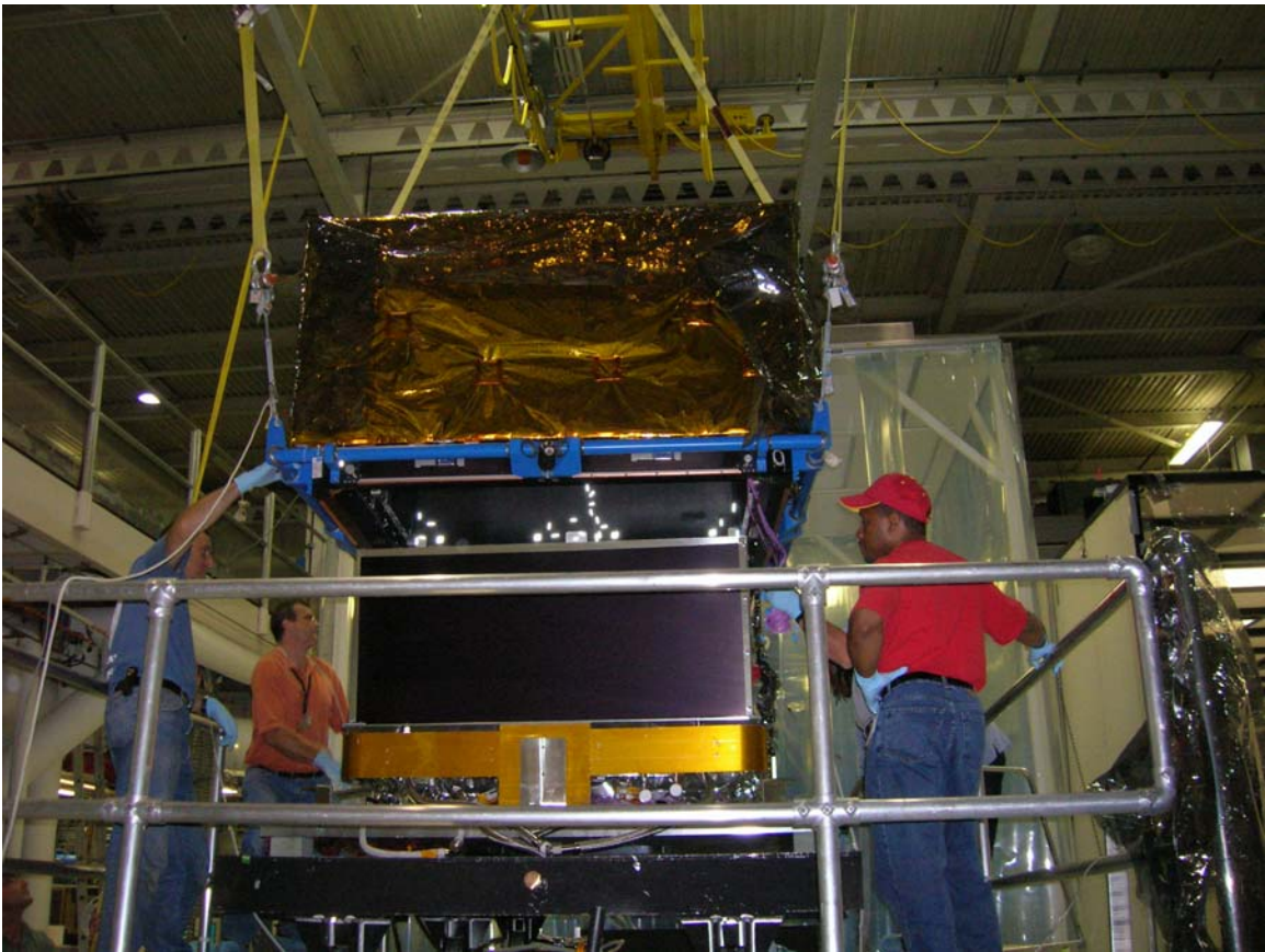
Figure K-2 - ACD installed on Thermal GSE
